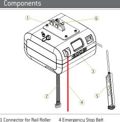
1 Connector for Rail Roller 5 Hand Control 2 Lift Belt **3** Secondary Panel 6 Mounting Pins
